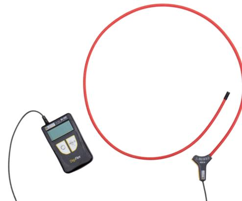
With its sensor 1 metre long, the **MA400D-1000** is designed to complete the electrician's toolkit for measuring or detecting leakage currents in the case of multi-conductor feeders requiring a large clamping capacity.
