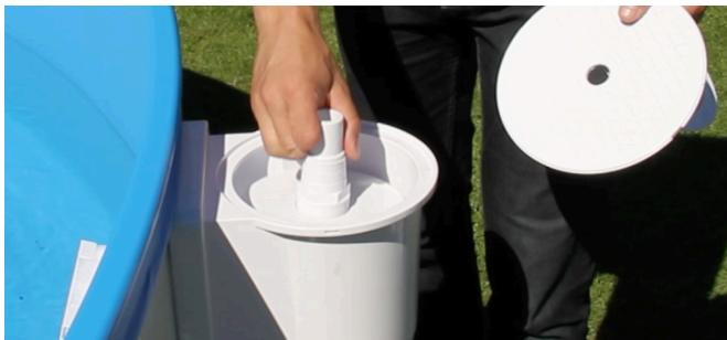
When vacuum-cleaning the pool floor, you can fit a hose to the filter system via the skimmer suction plate (6). Fit the pool hose to the suction plate using the elbow hose connector (7)(included).
