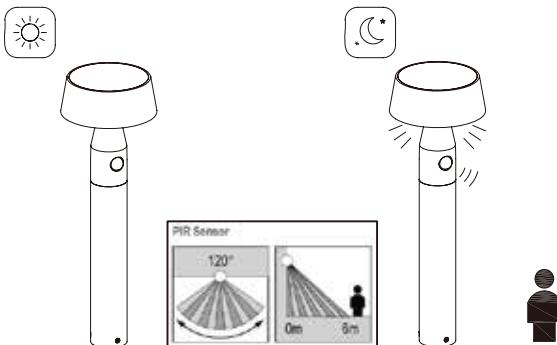
**ON :** (1) The light will constantly output 65lumen when the day light is less than 30LUX.
