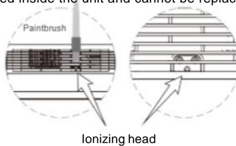
If crackling noises occur during operation, you should clean the head (as described in the picture) from dust with a narrow paintbrush.
