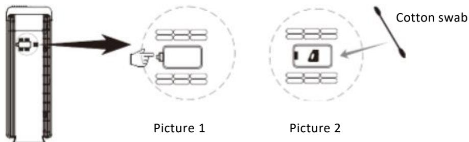
To do this, open the side flap (Fig. 1) and carefully wipe the sensor clean with a cotton bud
