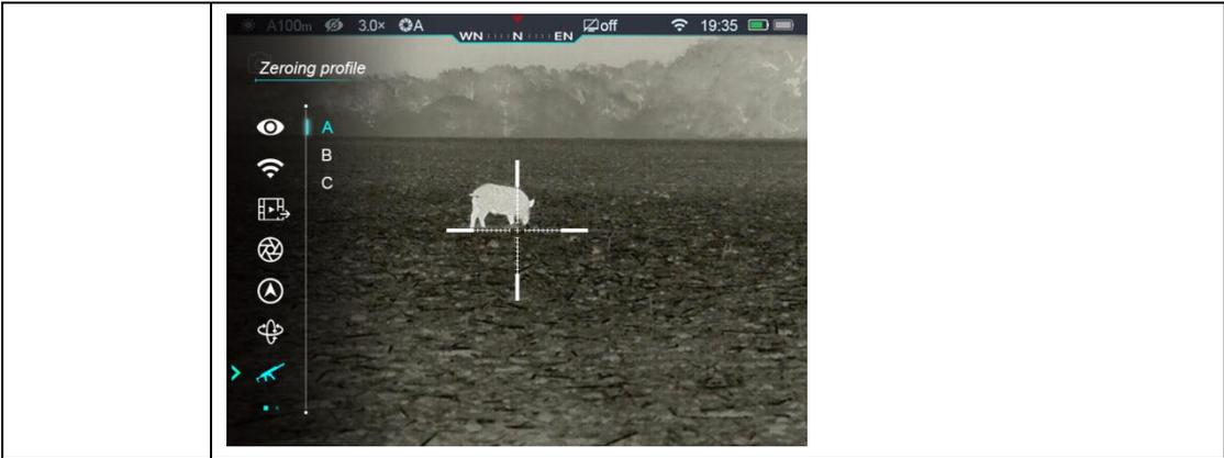
To zero your riflescope, you need to set a zeroing profile and zeroing distance first. Tube series support the zeroing distance in the range of 1 to 999 m.
