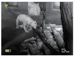
Picture-in-Picture improves accuracy by providing a 2x magnified image of the reticle area at the top of the display. It helps to zoom in on a target while retaining the rest of the field of view visible.
