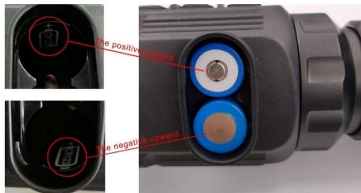
Fig. 8-1 Schematic diagram of battery installation
