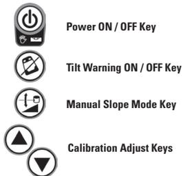
RL HV / RL HVPW / RLHVPW-G (See Figure ④)
