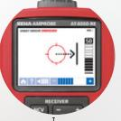
Large color display guides you in the direction and orientation of the energized wire.
