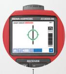
The Smart Sensor™ indicates that it is aligned with the energized wire. The display indicates the wires precise direction and orientation.
