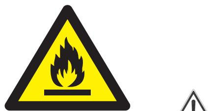
Flammable material. This appliance contains R290/Propane a flammable refrigerant.
