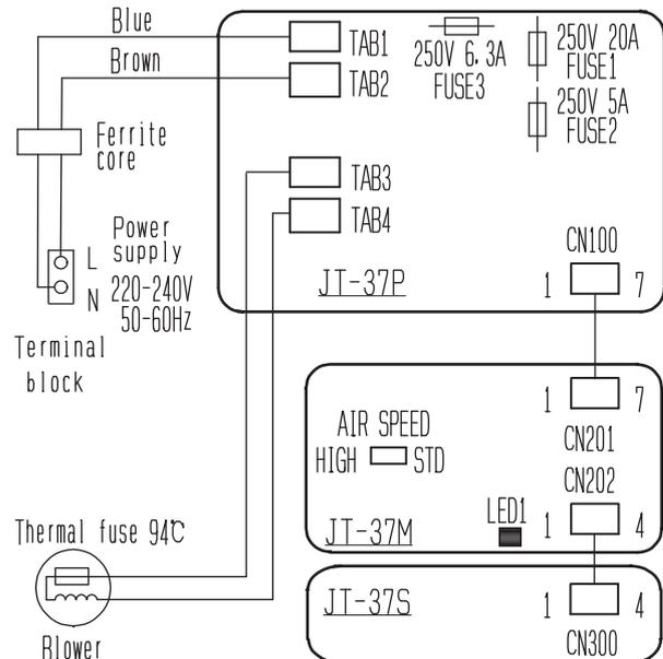
Current fuse in control circuit
