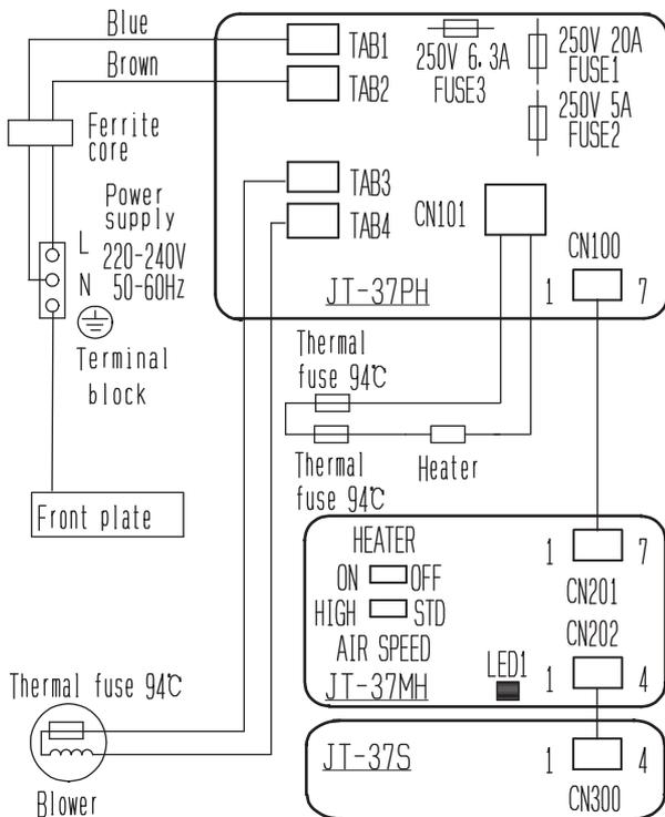
Current fuse in control circuit
