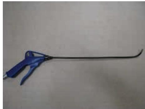
Clean with compressed air. Use a suitable nozzle.
