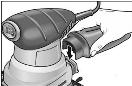
2. Periodically remove dust container from flange and empty collected dust.
