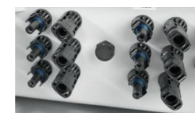
Image 3: Box with Weidmüller WM4 C connector; in the middle: pressure compensation element
