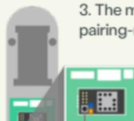
*Pairing-mode is indicated by slow flashing on both the blue and orange LED.*
