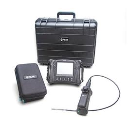
The Articulation Combo (Wired), Long Focus kit includes the VS70, a wired handset, and a dedicated 6 mm long-focus camera with two-way articulation on a 1 m semi-rigid cable. Long focus provides an increased viewing distance, and articulation provides greater internal camera control.
