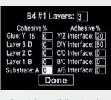
Record the pass/fail result and the nature of fracture - cohesive, adhesive, and glue failures - using the app (left) or the instrument's touch screen display (above)
