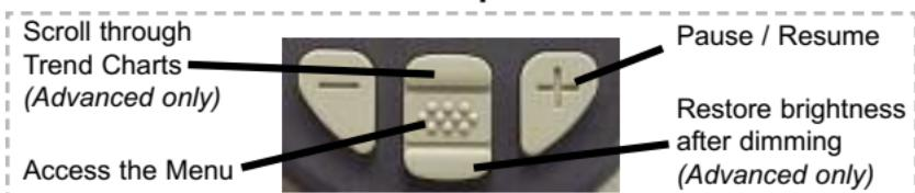
The Pause/Resume (+) button stops values from automatically updating to allow for closer examination of the relationship between the values or to allow time to manually record the entire dataset. Press (+) again to resume.
