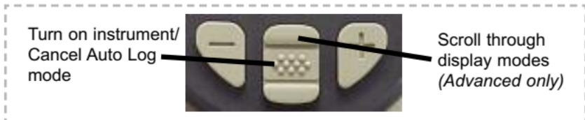
**Standard models** remain powered-up while in auto log mode. The instrument will take readings for 40-50 hours on a set of alkaline batteries, depending on the frequency of measurements.
