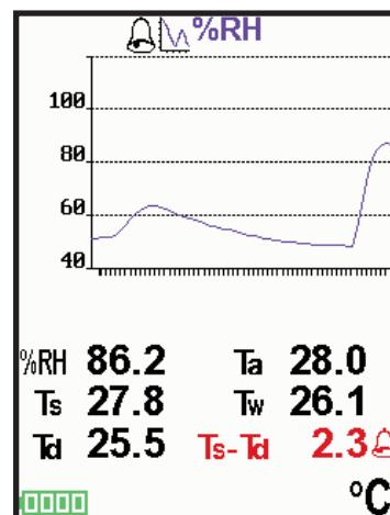
In alarm mode, if an alarm condition is met, the relevant reading is displayed in red, and the Alarm icon
