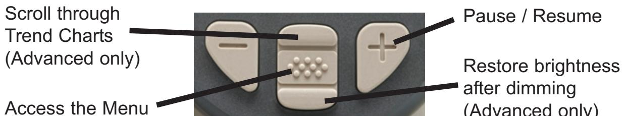
The Pause/Resume (+) button stops values from automatically updating to allow for closer examination of the relationship between the values or to allow time to manually record the entire dataset. Press (+) again to resume.
