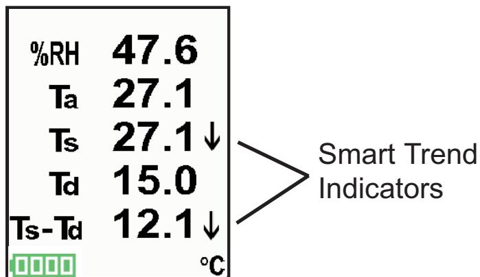
While the absence of an arrow does not necessarily signify stability, it can be taken to mean that particular reading is undergoing little or no change. Slow changes could therefore occur without being noted by an indicator arrow.
