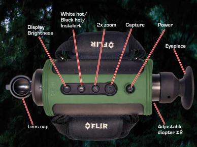
**Power Button** – The Scout camera has 3 power modes: On, Off, and Standby.
