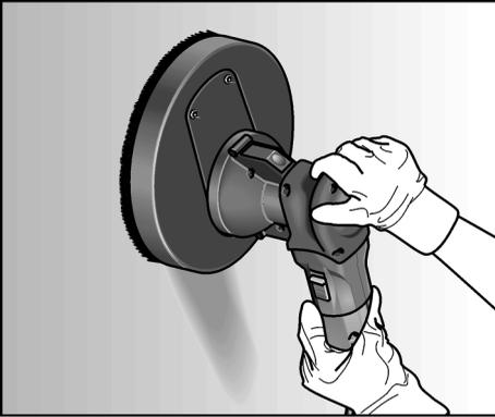
7. Grip the wall sander by both handles. Press the wall sander gently against the work surface (the pressure should be just enough to ensure that the sanding head is flush with the work surface).
