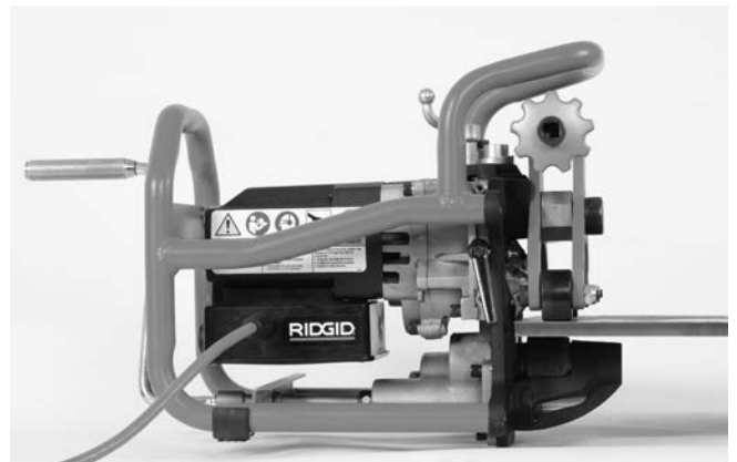
Figure 16B – Installing Beveller on Plate
