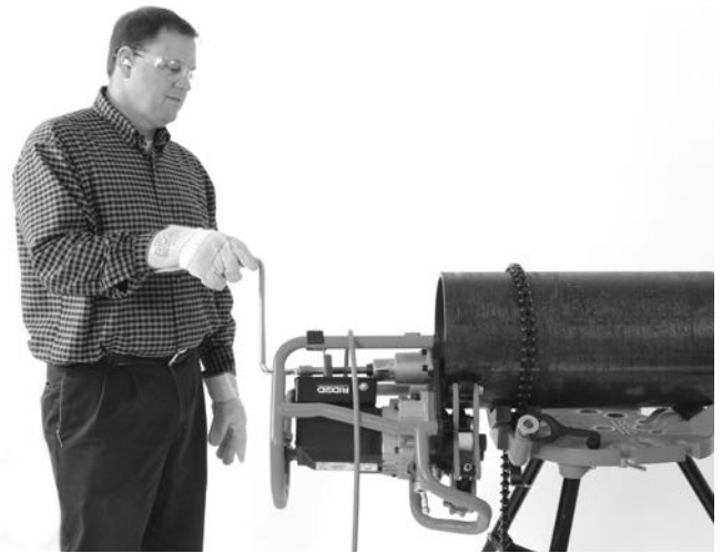
Figure 20B – Bevelling Operation (Fixed Workpiece/Moving Beveller)
