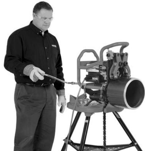
Figure 20C – Bevelling Operation (Fixed Beveller/Rotating Pipe)
