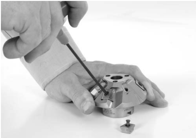
Figure 24 – Replacing Cutter Inserts
