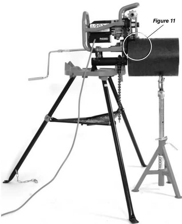
Figure 12 – Machine fixe, tuyau court, un porte-tubes
