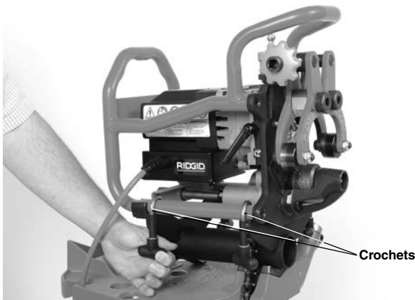
Figure 9 – Securing Beveler to Adapter
