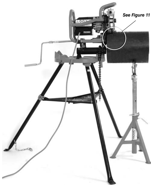
Figure 12 – Fixed Beveller, Short Pipe, One Pipe Stand
