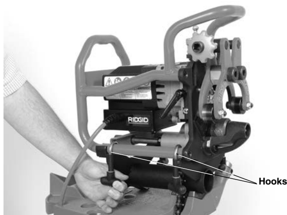
Figure 9 – Securing Beveller to Adapter
