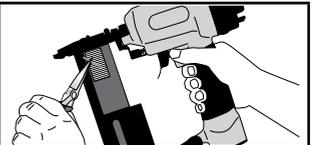
**MAINTENANCE:** While tool is disconnected from air supply, make daily inspection to ensure free movement of safety yoke and trigger.
