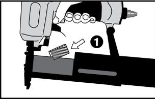
1. Loading staples: Place a strip of over the rail. Push the rail until it clicks into place.
