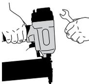
Disconnect tool from air before doing tool maintenance, clearing a jammed fastener, leaving work area, moving tool to another location, or handing the tool to another person. Never use tool if safety yoke, trigger or springs have become inoperable missing or damaged. Do not tamper with or remove safety yoke, trigger or springs.
