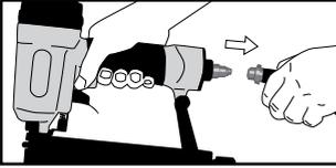
Disconnect the tool from air supply.
