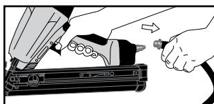
Disconnect the tool from air supply.
