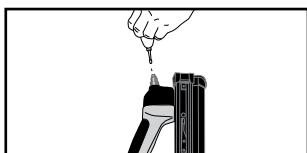
Squirt oil lightly with 2 or 3 oil drops into the air inlet. Only use supplied oil for the tool or recommended oil in the technical specifications.
