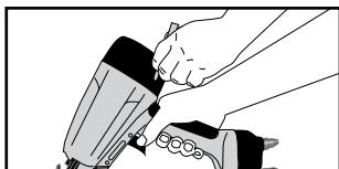
All screws should be kept tight. Loose screws result in unsafe operation and parts breakage.
