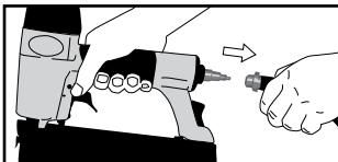
Disconnect the tool from air supply.
