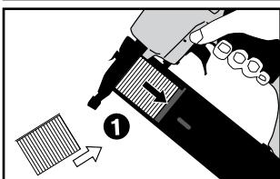
Loading brads: Hold the nail gun downwards and load a strip of nails into the cartridge, with the points facing downwards. Push the rail until it clicks into place. Use only recommended fasteners (see technical specifications).
