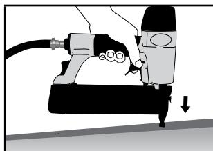
Keep tool pointed away from yourself and others and connect tool to air supply. Tools shall be operated at the lowest pressure needed for the application. This will reduce noise levels, part wear and energy use. Press the nose of the tool onto the workpiece to be fastened and press the trigger to fire staples. Adjust the mini pressure which is necessary for the penetration of the fasteners. Then, make some tests in starting with the lowest pressure.
