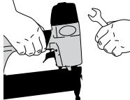
Disconnect tool from air before doing tool maintenance, clearing a jammed fastener, leaving work area, moving tool to another location, or handing the tool to another person. Never use tool if safety yoke, trigger or springs have become inoperable missing or damaged. Do not tamper with or remove safety yoke, trigger or springs.
