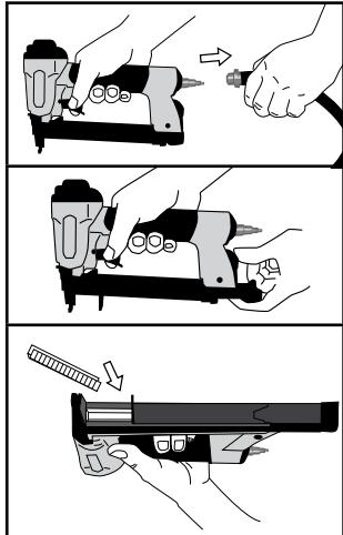
Disconnect the tool from air supply.
