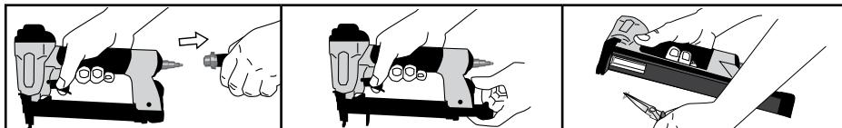
**MAINTENANCE:** While tool is disconnected from air supply, make daily inspection to ensure free movement of safety yoke and trigger.
