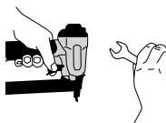
Disconnect tool from air before doing tool maintenance, clearing a jammed fastener, leaving work area, moving tool to another location, or handing the tool to another person. Never use tool if safety yoke, trigger or springs have become inoperable missing or damaged. Do not tamper with or remove safety yoke, trigger or springs.
