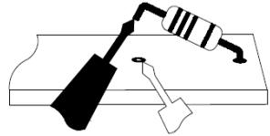
Fig. 5-7 Disconnected component
