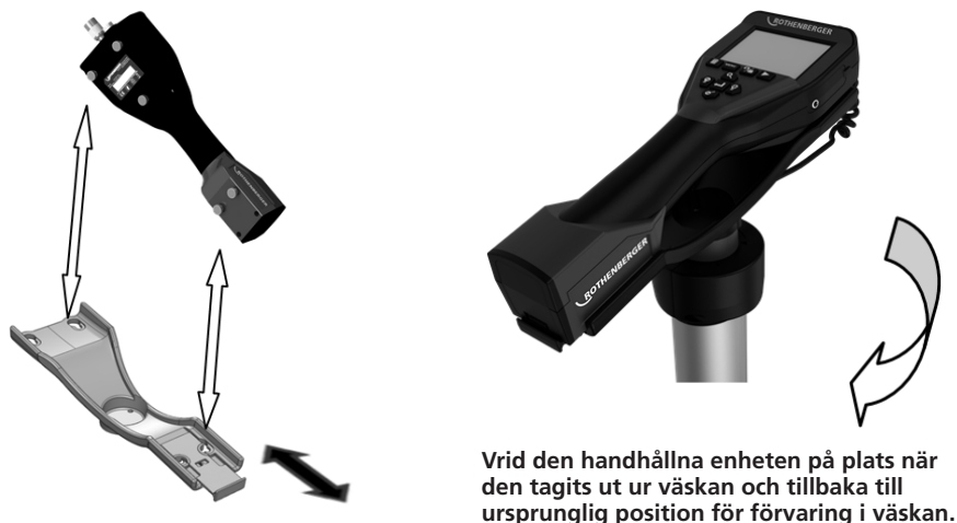
Figur 4 - Installing ROSCOPE 1000/i2000 handheld unit to the mounting cradle
