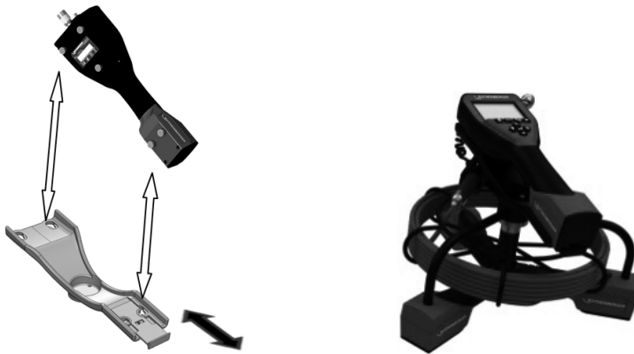
Figure 6 - Installing ROSCOPE 1000/i2000 handheld unit to the mounting cradle
