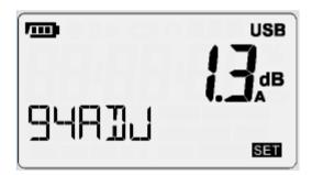
Press the Enter  $\stackrel{\bigodot}{\bigodot}$  key to save the entry and to get back to the measure window. The meter should now read 94.0dB (+/- 0.1dB).
