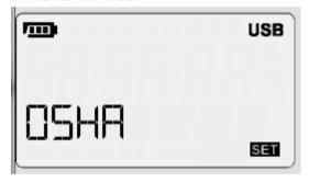
Press the or v button to select a NDM testing regulatory body abbreviation: OSHA, MSHS, DOD, ACGIH, ISO85, ISO90, and USER.
