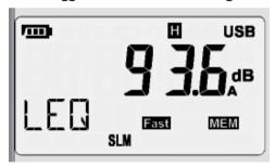
For Sound level readings, SLM must appear on the lower line. Press and hold the mem button for more than 1 sec to enter the viewing mode. Press the or button to scroll through the readings.
