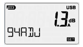
Press the Enter key to save the entry and to get back to the measure window. The meter should now read 94.0dB (+/- 0.1dB).
