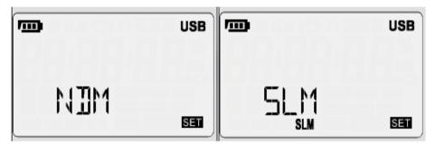
Press the or volume button to change the test mode between NDM (Noise Dose Meter) and SLM (Sound Level Meter).
