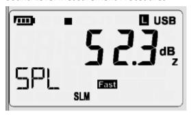
Press the button to turn on the meter. The LCD will display the **SPL** symbol, with SLM on the lower line. If SLM is not visible press SET and NDM will appear, press the Down arrow to change to SLM and press enter to exit.
