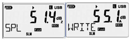
Press the button to enable the auto data record function. The REC symbol will flash on the LCD display. The bottom left of the LCD display will show **WRITE**, at each sample interval to indicate that the data was written to the meter's internal memory.
