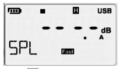
Press the button to turn on the meter. The LCD will display the SPL (sound pressure level icon). If SLM is showing in the lower line, Press SET and press the down arrow to change SLM to NDM. Press the Enter button to exit setup. Press the button to enable noise dose testing. Press the button again to pause testing. Press
