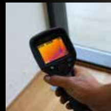
Find air infiltration problems
