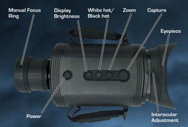
**Power Button** – The BHS-Series Bi-Ocular camera has 3 power modes: On, Off, and Standby.
