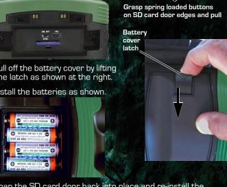
5. Snap the SD card door back into place and re-install the battery cover—it only fits one way.
