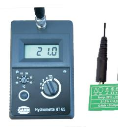
Examples for checking of the Hydromettes HT 65 and BL H 40 using the mesuring cable MK 8 (order code 6210)
