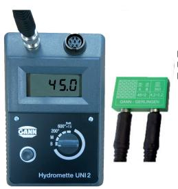
Examples for checking the Hydromettes UNI 2 and BL E using the measuring cable MK 8 (order code 6210)
