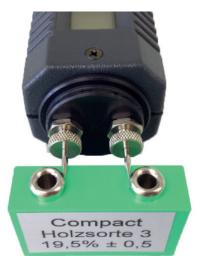
Compact meters can be checked, too. Hold the pins against the socket as shown in the pictures. The pins must touch the sockets.
