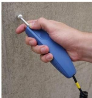
The hand of the operator influences the measurement field of the ball electrode and changes the measured value as it is shown in figure 4-2.
