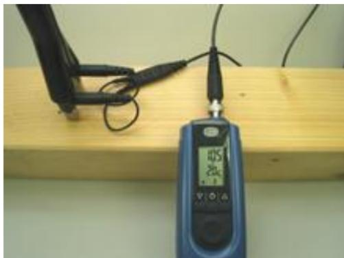
Figure 4-3 Measuring across the fibre direction with M 20
