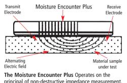
principal of non-destructive impedance measurement. Coplanar electrodes are fitted on the base of the instrument from which low frequency signals are transmitted into the material being tested, measuring the change in impedance caused by the presence of moisture. This reading is translated by the instrument into a moisture content reading.
