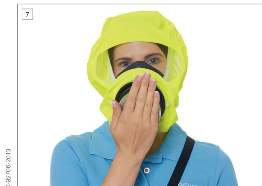
Check the fit of the half mask by closing the front filtering opening with the palm of your hand. If negative pressure is not generated readjust the half mask to ensure a close fit over nose and mouth.
