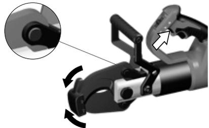
2. Remove the battery pack and pull the slide switch in position lock.
