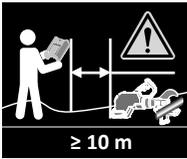
If no national or other requirements exist, the appropriate minimum distances in air, which define the outer limits of the danger zone or the approach zone, can be found in the most recent version of the European Standard 50110-1. The manufacturer's recommendation is  $\geq 10\text{m}$
