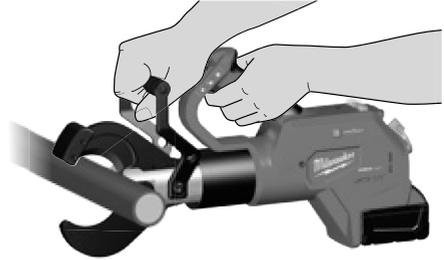
2. Grasp handle(s) firmly. Move the slider switch into the unlocked position. (1)
