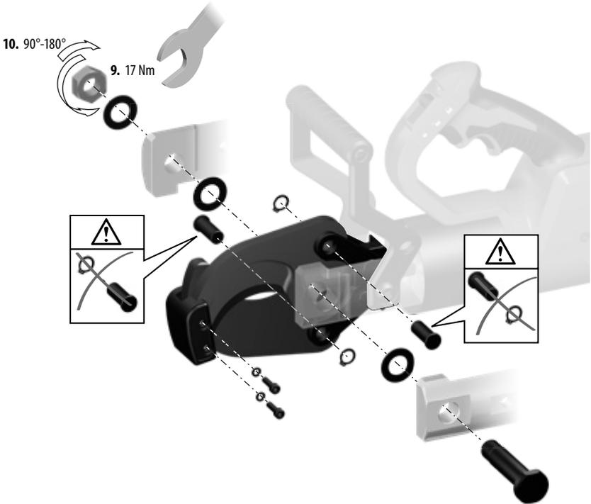
1. Use a wrench or pliers to remove the blade nuts and remove the blade bolt.
