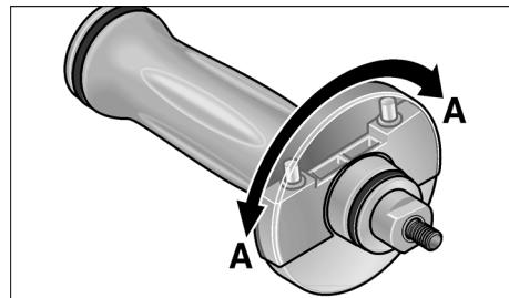
3. Rotate the cover on the handle by 180° until it engages.
