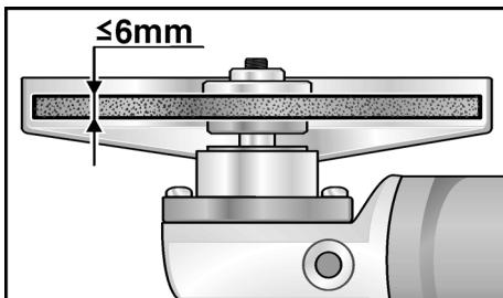
7. Screw the clamping nut (3a), with flange face up, onto the spindle.
