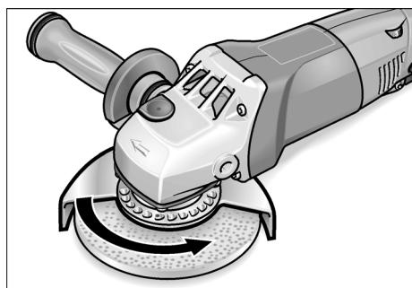
2. Rotate the safety guard (4a) away from the direction-of-rotation arrow on the gear head (7) until it is in the required position.
