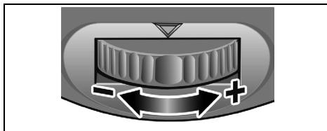
To set the stroke number, move the thumb wheel to the required value.
