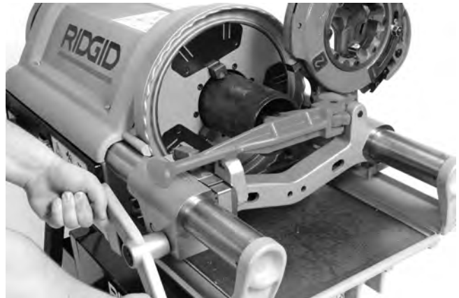
Figure 22 – Reaming Pipe with Reamer
