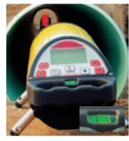
Automatic grade compensation with the housing rolled up to  $\pm 3^{\circ}$ , the Piper will compensate and correct for the grade errors.
