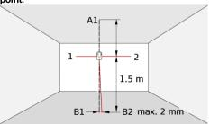
Rotate the instrument by  $180^{\circ}$  so that it points in the opposite direction 2 to direction 1. Adjust the instrument so that the laser beam hits point A1 exactly. If point B2 is no further than 2 mm away from point B1, then the Leica Lino is within tolerance.
