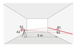
Then place the instrument at the same elevation as close as possible to wall A and again mark the horizontal laser line or the laser point on wall A (A2). Rotate the instrument by 180° again and mark the laser on wall B (B2). Measure the distances of the marked points A1-A2 and B1-B2. Calculate the difference of the two measurements
