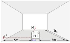
Place lock switch in "Unlocked" position (see Levelling lock). Mark a reference point (P1) approx. 5m from the walls and position the lower plumb point exactly on it. Align the cross hair to the left wall and mark the intersection point (a1) approx. on the same hight like P1 to the wall. Shortly after mark the right-hand perpendicular beam (b1) on the front wall
