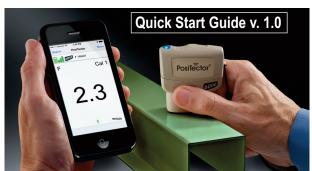
Wirelessly connect PosiTector probes to your smart device
