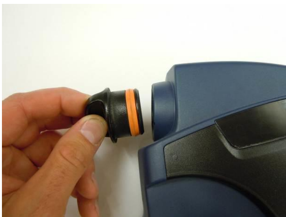
Assemble the third plug with gasket into the air outlet of the fan unit.
