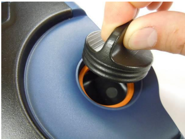
Turn in the threaded plugs into the filter inlet.
