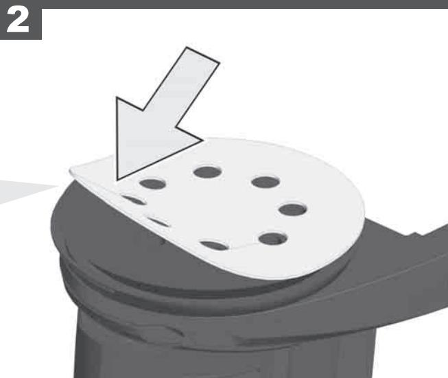
Press carefully the fuzzy side of sanding disc against the packaging pad, as firmly as possible.
