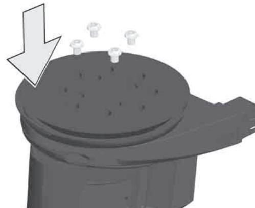
Replace sanding base if hook&loop material is worn out.
