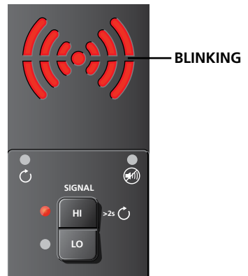
Figure 3.1c: Transmitter screen showing signal in HIGH mode
