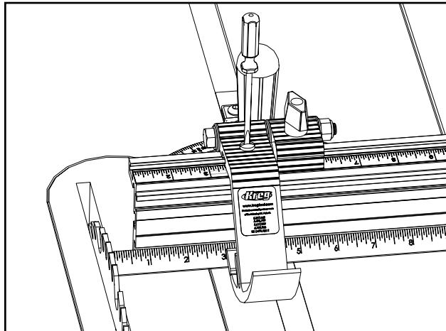
Use a steel shop ruler (one with the zero mark flush with the end) to position the stop arm 3" from the blade. Let the blade teeth graze the end of the ruler. (Do not use the cursor and measuring tape to position the stop arm.) Tighten the stop T-knob.
